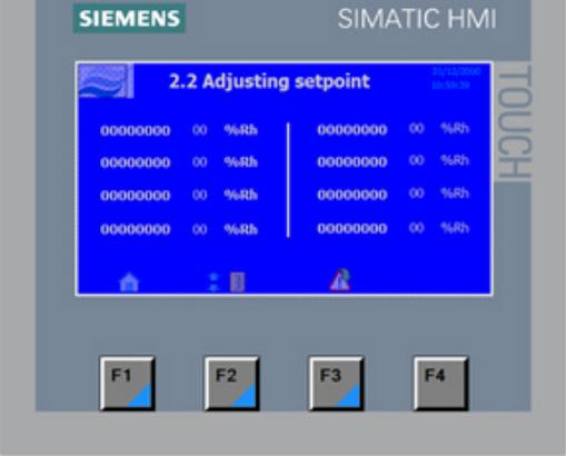
Force the HP pump to run by adjusting the set point in a section to 75%.
